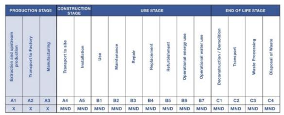
Figure 1 Production stage system boundary
