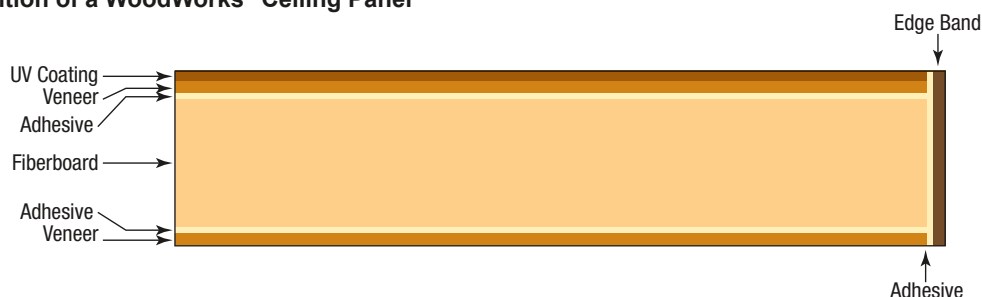
Figure 1. Composition of a WoodWorks® Ceiling Panel
